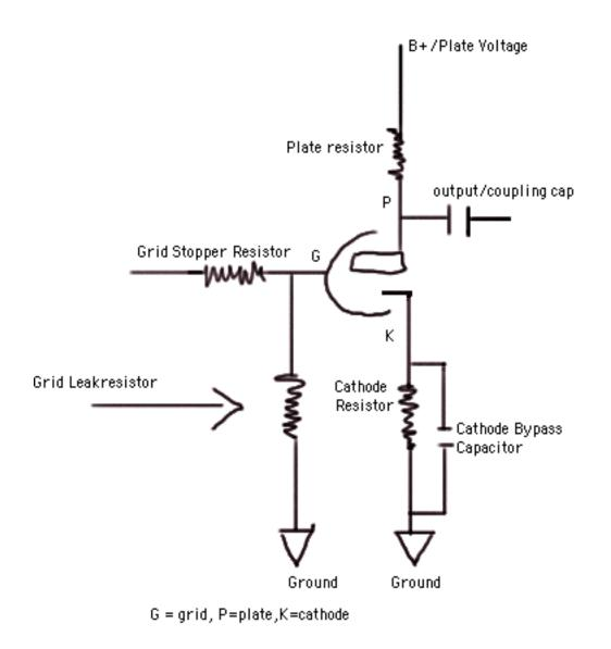
The grid ("leak") resistor,
