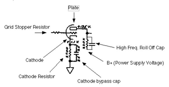
"Complete" typical tube preamp stage:
