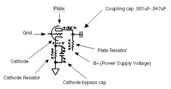
Another modification you may see is a Grid Stopper Resistor, this can also control gain between stages and also interacts with the tube to roll off highs. Values can be 1.5K->100K. Larger values roll off more highs and reduce gain between stages. The Grid Stopper Resistor works best when mounted directly or as close as possible to the grid pin. DIYstompboxes.com » Tubes for dummies
